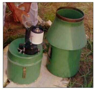
Figure 2.1: Installation of natural siphon recording rain gauge
