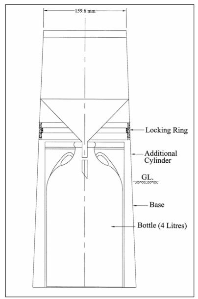
Figure 1.1: Standard rain-gauge
