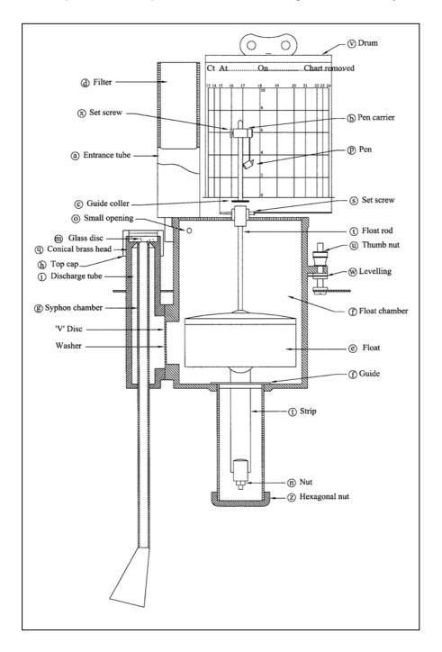
Figure 2.2: Recording mechanism of autographic rain gauge
