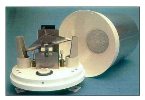
Figure 3.1: Tipping Bucket rain gauge
